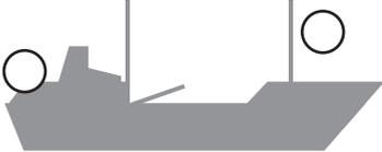
Power driven vessel over 50 metres at anchor
